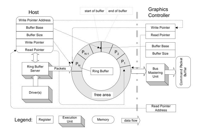
Figure: Ring Buffer and its Control Structure
